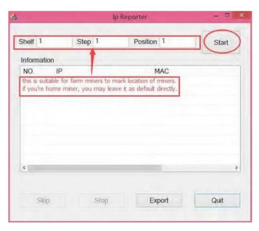
7. On the control panel, click the IP Report button. Hold it down until it beeps (about 5 seconds). The IP address will be displayed in a window on your computer screen.
