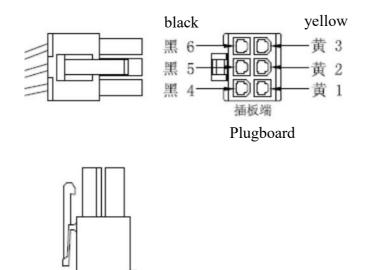
The output cable consists of two colors: the 12V positive terminal is yellow; the negative terminal is black
